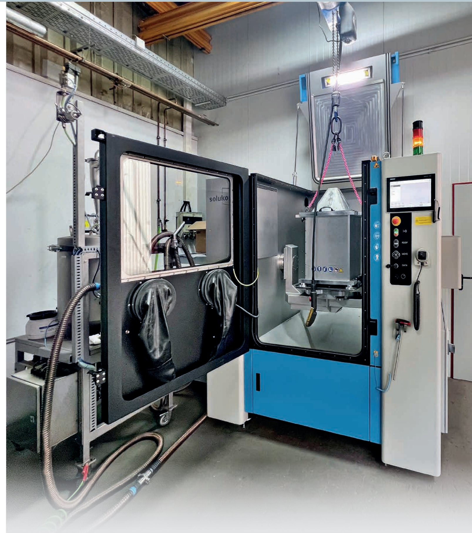
The building box with component and powder is unloaded from the Reichenbacher printer and inserted into the Solukon system. There, the box is turned upside down first as a whole before (after removal of the frame) fine cleaning takes place without the box.
