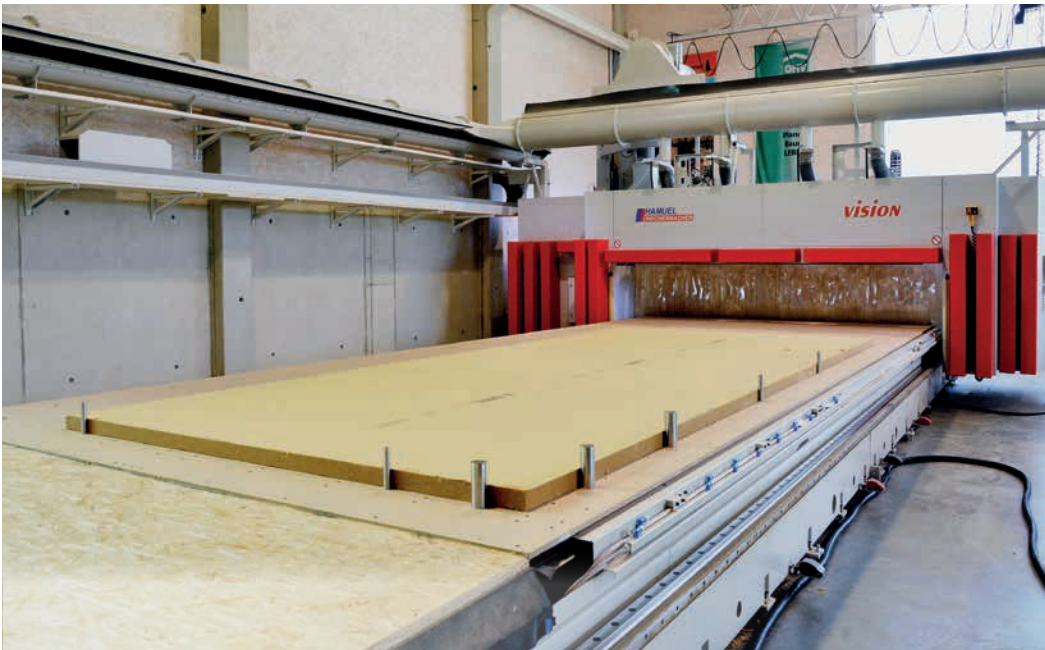
Processing table with special table extension and stops.
