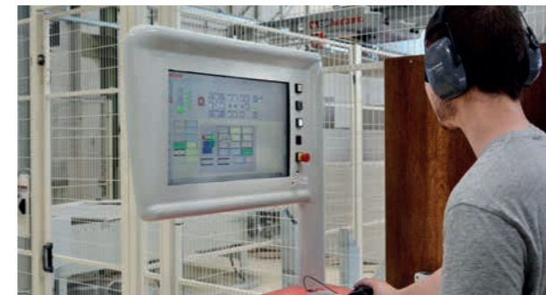
A central CAD planning system provides the complete data sets with the correct project reference directly to the respective workstation.
